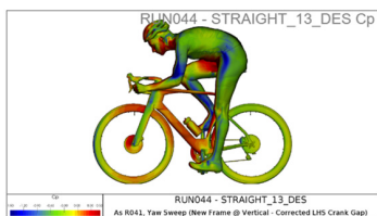
Step three - Optimisation of the head tube/top tube transition.
